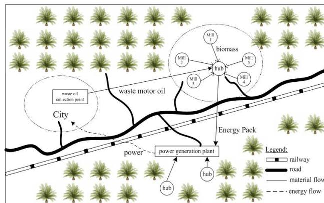
Figure 1: The concept of biomass processing hub and material/energy flow of proposed energy strategy
