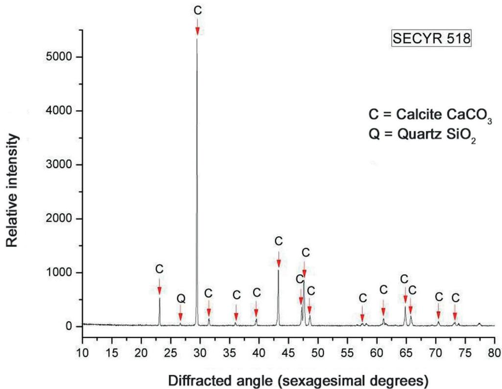
Figure 7. X-Ray diffractogram theta/2theta of sample No. 2, MAEF 10013/69/23.
