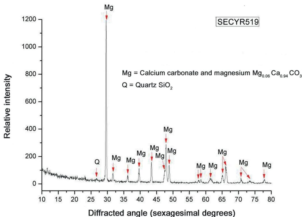
Figure 8. Grazing Incidence diffractogram of sample No. 3, MAEF 5128.
