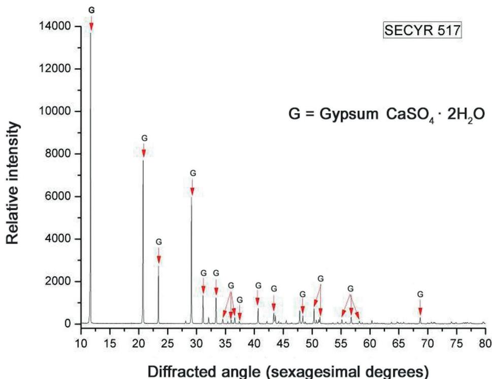
Figure 6. X-Ray sweep powder diffractogram theta/2theta of the stone vessel MAEF 2631.
