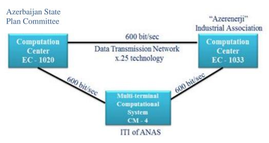
Figure 1. Data Transmission Network based on x.25 technology.
