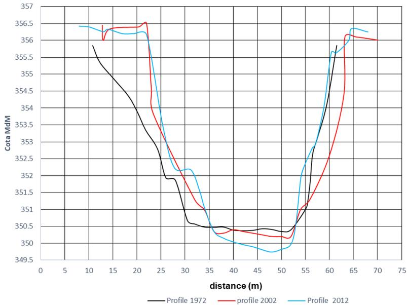
**Fig. 4. Transversal profiles of the riverbed in the section of Bistrita hydrometric station**
