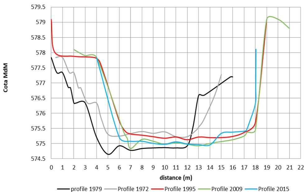
**Fig. 2. The transversal profiles of the riverbed in the section of the Bistrița Bârgăului hydrometric station**
