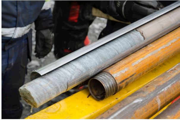
Fig. 9.4: The first drill core (bedrock in the lower part, cement in the upper part) was pushed out of the inner tube of a triple tube core barrel assembly. Clearly visible is the split aluminium liner that protects the drill core from external forces. The second tube is also called core barrel, and the third tube is the drill string, hence “triple tube”.
