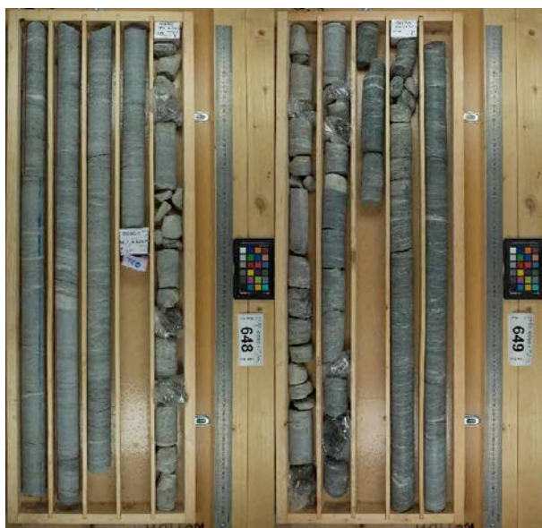
Fig. 9.2: Core boxes 648 and 649 from COSC-1. The core boxes are used in portrait format (=upper left corner = Top, lower right corner = Bottom. Top and bottom of core runs are marked with labelled foam blocks. Each box was photographed with the cm/ft ruler and a standard colour chart.
