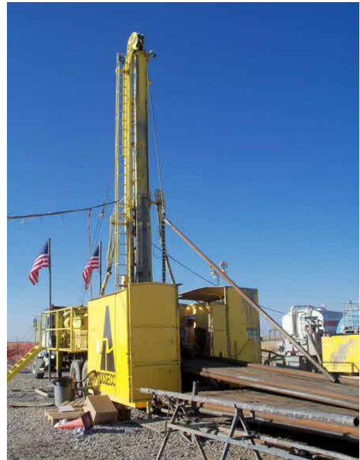
Fig. 4.2: Truck-mounted wireline coring rig of DOSECC of HOTSPOT project
