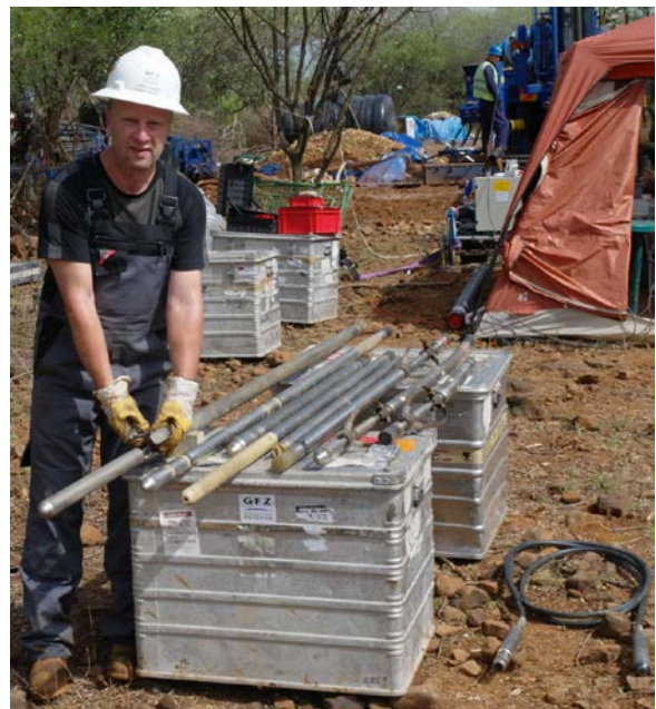
Fig. 6.3: OSG slimhole logging sondes at drillsite
