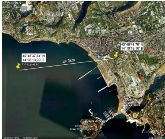
Fig. 4.8: Horizontal well trajectory for the Campi Flegrei deep drilling project in Italy
