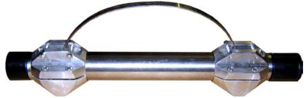
Fig. 7.4: Spring bow de-centralizer hole lock concept (photo: SAFOD project)
