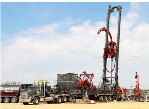
Fig. 7.3: Coiled tubing operation from a flat-bed truck with truck-mounted derrick
