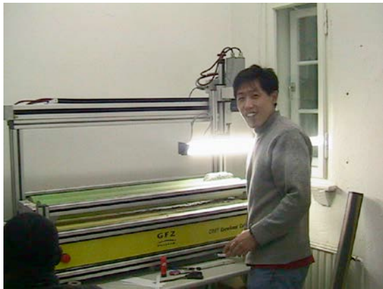
Fig. 8.2: Optical core scanner in operation
