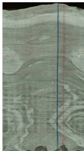
Fig. 9.1: Whole round core scan of core section showing double reference line in upright position with red line on the right (COSC project)
