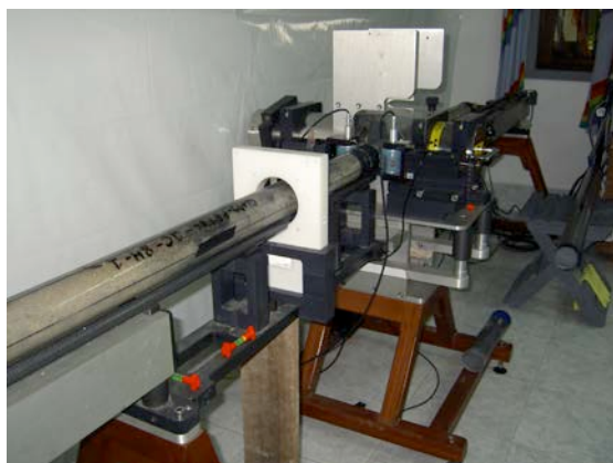
Fig. 8.1: Multi-sensor core logger in field lab
