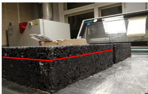
Fig. 5. BBTM 11 is compacted on top of AC22 base course
