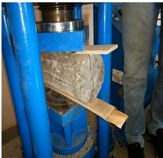
Fig.3.28 Testing cylindrical concrete specimen
