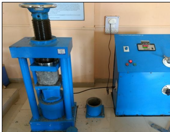
Fig 3.20 Compression Testing of cubes
