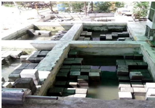
Figure 2- Casting of cubes and curing tank
