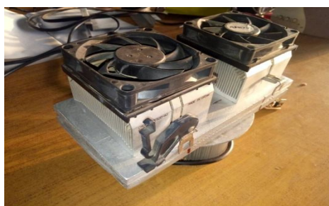
Fig: 6 Experimental Setup using a thermoelectric modules model TEP1-1264-1.5 Between a Controlled hotplate and a cooling fan
