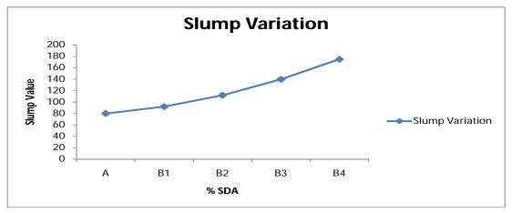
From these results it was notified that concrete becomes more workable as PEG-400 %age is increased that means less water is required to make mix more workable.
