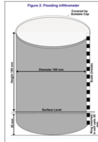
The area enclosed in the ring has flooded with water and the time required for one centimeter of water to infiltrate have been measured. The ring has covered for reduction of evaporation losses during the test. Measurements have been continued until the rate became more or less constant or starts rapid lateral spread of water.
