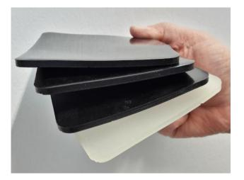
Figure 2. Biopolyurethane samples. Mass proportions (%) of Sphagnum moss (from top to bottom): 16, 10, 4, and 0 %.
