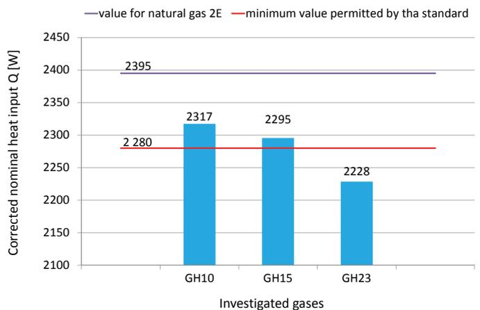
**Fig. 5.** Corrected nominal heat inputs for a balanced flue type air heater for space heating
