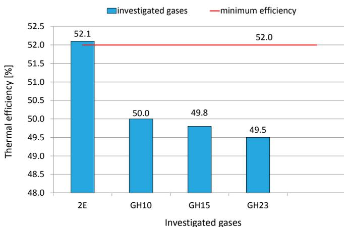
**Fig. 3.** Results of thermal efficiency for the burner of a gas stock pot range
