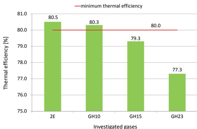
**Fig. 6.** Results of thermal efficiency for a balanced flue type air heater for space heating
