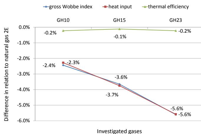
**Fig. 9.** Difference of gross Wobbe index, heat input and thermal efficiency values of investigated mixtures with hydrogen in comparison to natural gas for a gas-fired air heater
