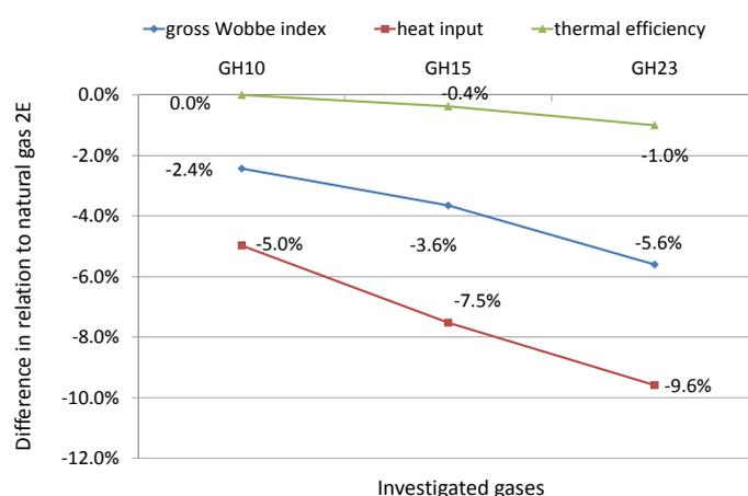
**Fig. 8.** Difference of gross Wobbe index, heat input and thermal efficiency values of investigated mixtures with hydrogen addition in comparison to natural gas for a gas fireplace
