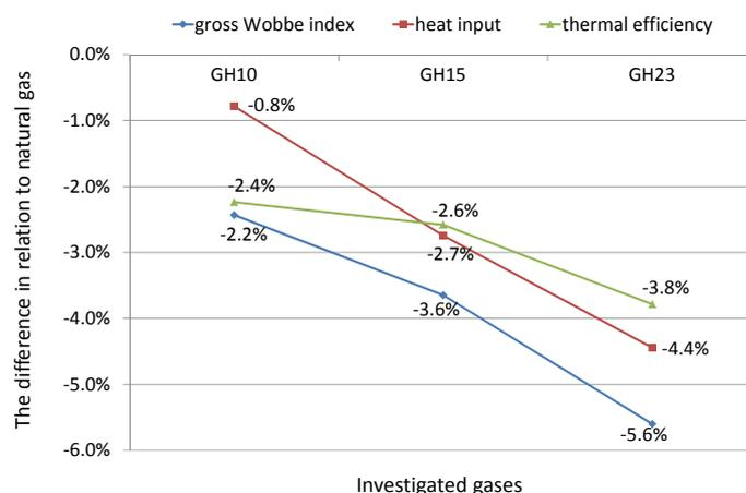
**Fig. 2.** The difference of gross Wobbe index, heat input and thermal efficiency of investigated mixtures with hydrogen in relation to natural gas of a semi rapid gas hob's burner
