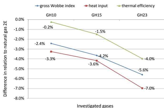
**Fig. 7.** Difference of gross Wobbe index, heat input and thermal efficiency values of investigated mixtures with hydrogen addition in relation to natural gas for a balanced flue type heater
