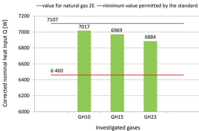
**Fig. 10.** Corrected nominal heat input for a gas-fired overhead luminous radiant heater
