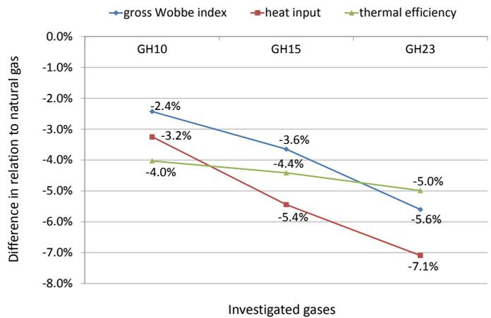
**Fig. 4.** Difference of gross Wobbe index, heat input and thermal efficiency of the investigated mixtures with hydrogen content in relation to natural gas 2E for a burner of a gas stock pot range
