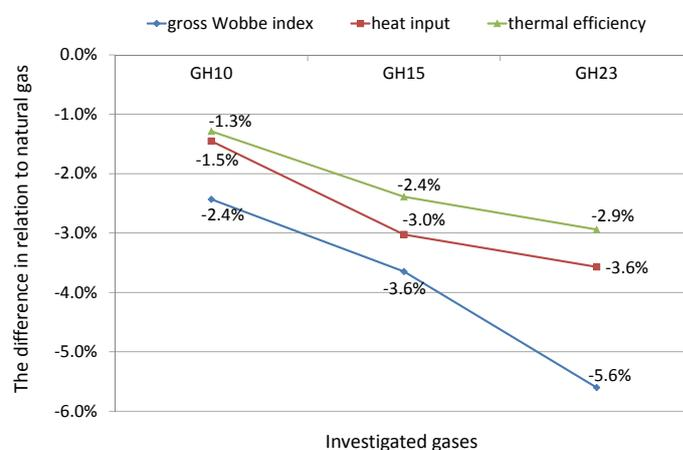
**Fig. 1.** The difference of gross Wobbe index, heat input and thermal efficiency of investigated mixtures with hydrogen in relation to natural gas of a large gas hob's burner
