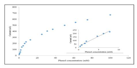
Figure 6. The dynamic calibration range of the sensor towards different concentration of phenol. Inset is the linearity range of the sensor
