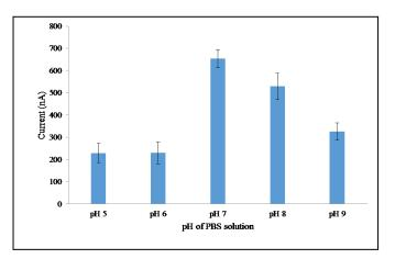
Figure 5. Influence of pH on the response of the immobilized tyrosinase in NCC/Chitosan composite film
