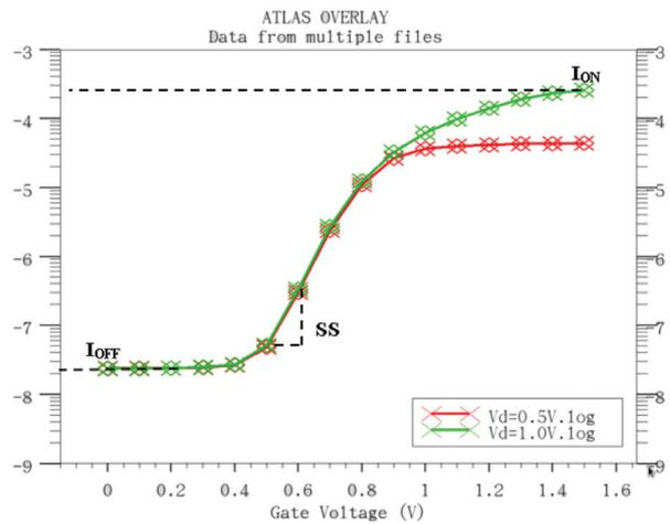
FIGURE 4. I<sub>D</sub>-V<sub>GT</sub> of GFET at different V<sub>D</sub> with I<sub>D</sub> in log scale
