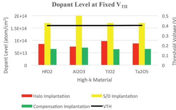
FIGURE 2. Factors variation of different dielectric material at fixed V<sub>TH</sub>
