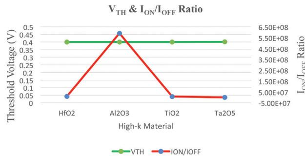
FIGURE 7. Results of  $I_{ON}/I_{OFF}$  at fixed  $V_{TH}$
