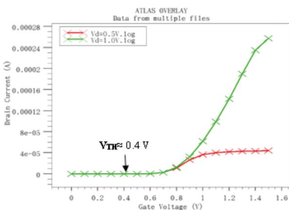
FIGURE 3. I<sub>D</sub>-V<sub>GT</sub> of GFET at different V<sub>D</sub>
