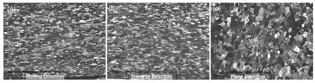
Figure 1: Microstructure of the AA2139-T351 alloy Slika 1: Mikrostruktura zlitine AA2139-T351
