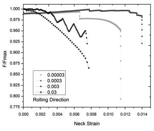
Figure 11: Rolling-direction loss of the load-carrying ability during the necking
