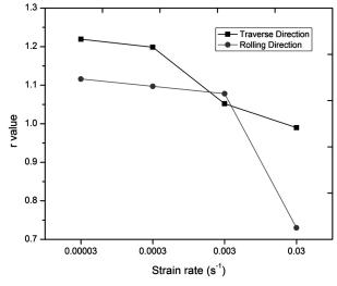
Figure 6: Anisotropy – strain rate relation Slika 6: Odvisnost: anizotropija – hitrost obremenjevanja
