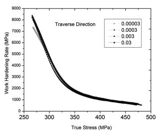
Figure 8: Work hardening rate – true stress relation in the transverse direction
