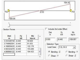
Fig 2- Shear bending of BEAM 1632
