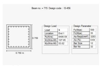
Fig 4- Concrete design of Column 715 in CASE 1
