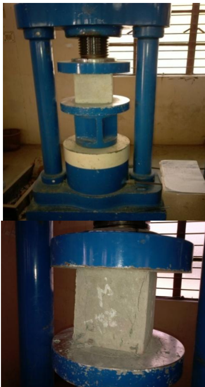
Fig-19 Compression test on cement mortar
