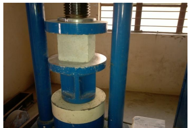
Fig-20 Compression test on concrete
