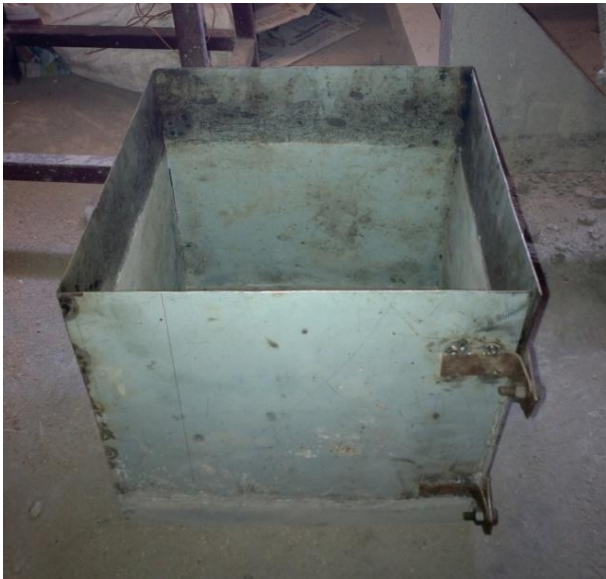
Fig-2: Prepared mould (27x27x20cm)
