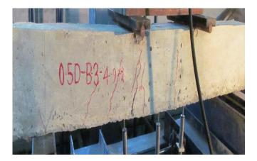
Fig.-10: The Crack Patterns of 0.5 Depth Level of Fiber RC beam Specimens
