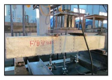
Fig.-7: Beam and LVDT arrangement in 1000 kN Loading Frame
