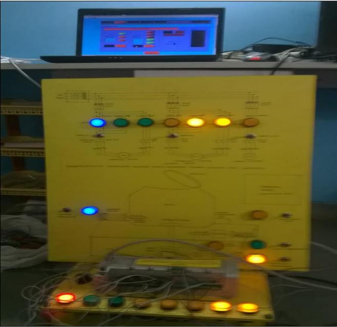
Fig -8: Computer running Lab View HMI with PLC Hardware
