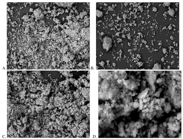
Fig.2. The SEM images of post-galvanized sewage sludge at the different magnifications: 100  $\mu$ m (A and B), 50  $\mu$ m (C), 10  $\mu$ m (D).
