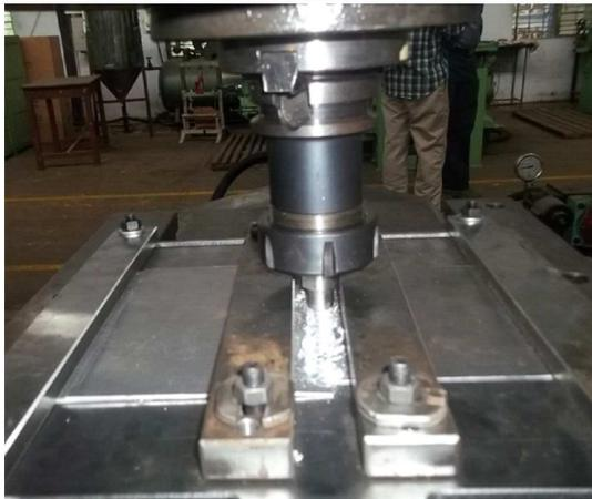
Fig. 4. Welding fixture with probeless tool.
