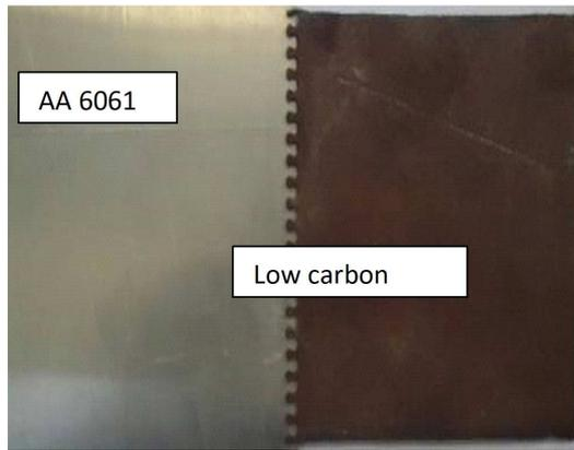
Fig. 3. Top surface of the joint.
